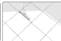
For dirty grout joints, scrub with a grout brush
