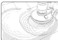
For larger areas use a slow speed scrubber;
