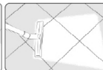
After scrubbing, remove with wet vac and rinse
